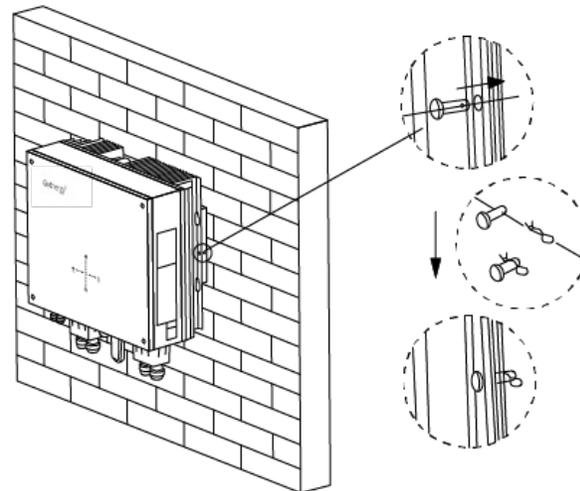
Brackets should be installed with the hooks pointing upwards and secured using the 4 fixings points provided.
