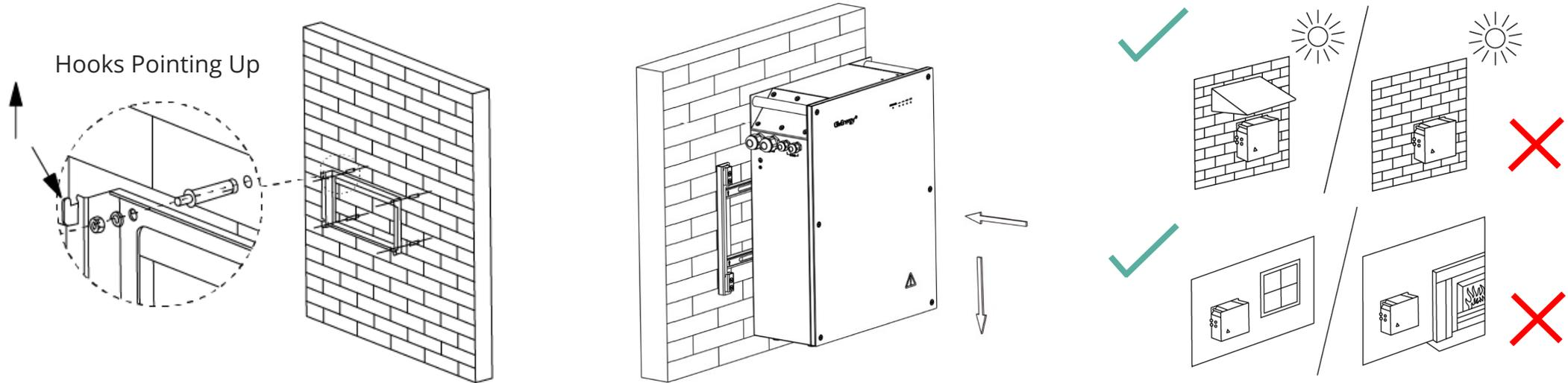
All batteries must be secured to the wall using the fixings provided, even if the weight of the battery is on the floor.
