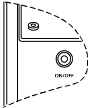
Isolate battery by pressing the On/Off switch on the side for 5 seconds
