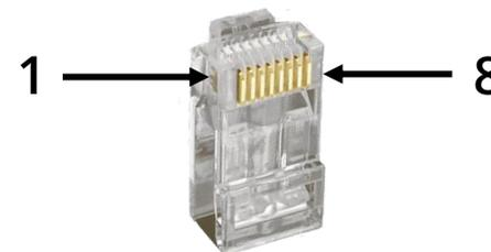
Data connections are identified by holding the locking tab of the RJ45 plug facing away from you and the terminals labelled 1 – 8 from left to right as pictured above
