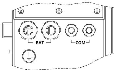
All batteries must be earth bonded together back to the inverter.
