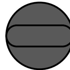
Turn off the PV with the external isolator first (if fitted) then the built in isolator
