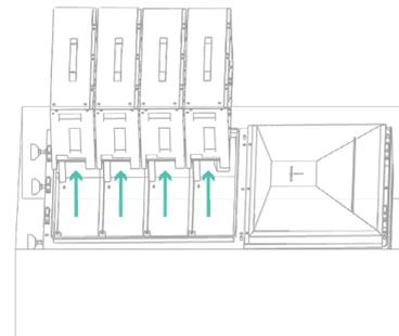
5. Remove the battery packs, leave to one side
