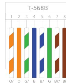
**Please note:** The communication cable must be terminated with a RJ45 plug at either end to connect the All in One to the Giv-Gateway. Ensure the wiring configuration into the RJ45 is the same both ends, a cross-over cable will not work. A standard Ethernet Cat5/6 cable will suffice here wired to T-568B standard if doing locally.
