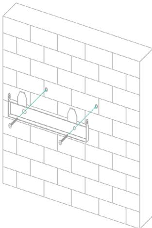
3. Fix the Giv-Gateway to the mounting bracket and secure with the fixings provided. Ensure there is adequate clearance space.
