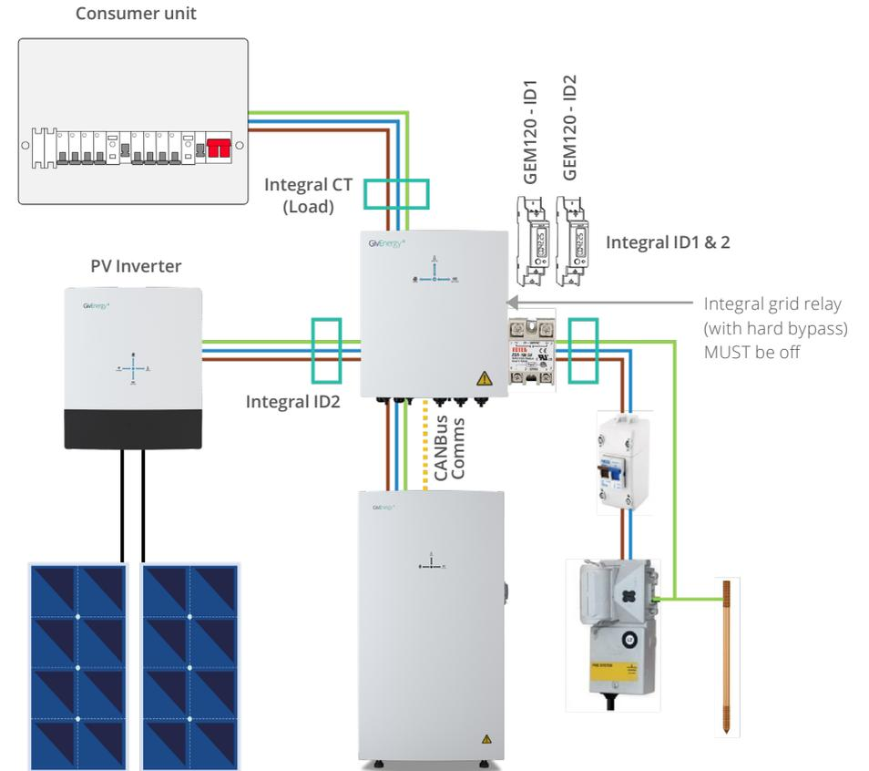
Note: An earthing rod **MUST** be installed.
