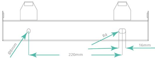
2. Fix the mounting bracket to the wall using the fixings provided, or other suitable fixings.
